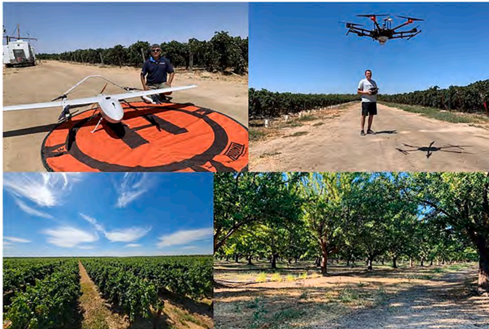
Fig. 9. Top row: Examples of the USU AggieAir drone technology used in the GRAPEX and T-REX projects, including (left) a custom hybrid fixed-wing drone with 1.5+ hour flying capabilities, and (right) vertical take-off and landing (VTOL) drone for surveying smaller areas. Bottom row: Example of the canopy structure in vineyards (left) and almonds (right) that UAV imagery can describe. Note the interrow conditions (with or without cover crop), tall, clumped canopy of the main crop, and the changes in interrow exposure to sunlight depending on sun angle and row direction.
