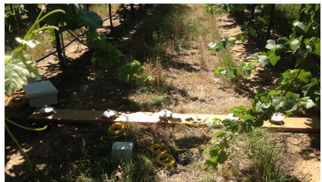
Fig. 5 A west-viewing photograph illustrating the variation of sunlit and shaded areas in the interrow of the south vineyard during June 2015 IOP. Note the sunlit areas illuminating the radiation sensors underneath the vines on the south vine row (left-hand side) and shading even in the center of the interrow
